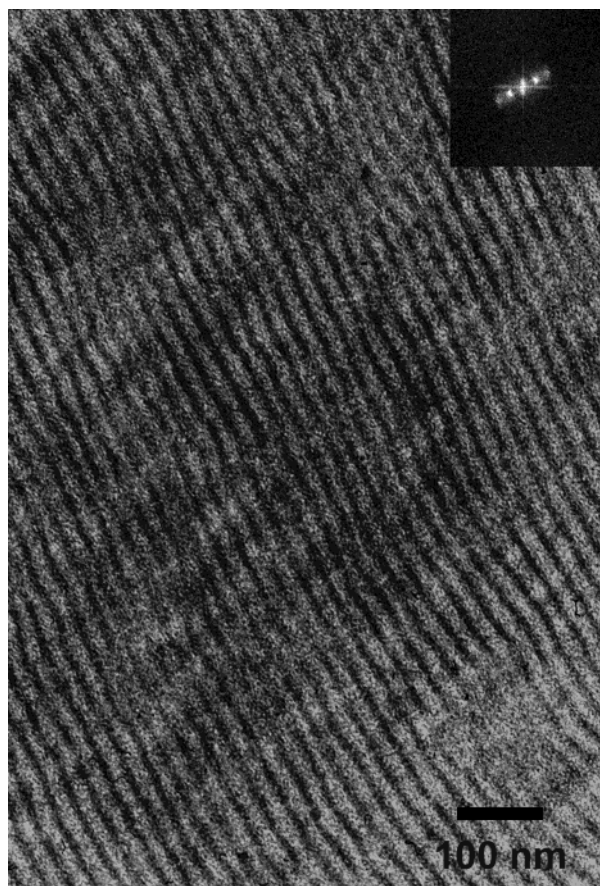
Figure 3. TEM micrograph of a thin section of PS 109 –PMPCS 41 . The sample was sectioned along the yz plane followed by RuO 4 staining for 30 min. The dark regions are PS domains, which were stained by RuO 4 .
